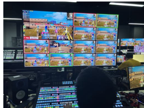
Fig. 4. The multi-screen view for the director. The largest screen on the left top of the screen is the current streaming video. Two screens on the right top are the PGM and PV. The rest of the screens receive the live video signals from the observers.
